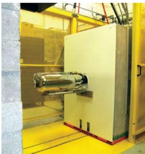
The D-T neutron generator mounted on the shielded door assembly. The door, weighing approximately 5 tons, is moved into and out of the irradiation position using air pads located beneath the door.
