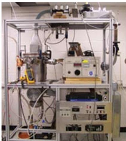
**Microwave plasma cathode experiment vacuum chamber and apparatus.**
