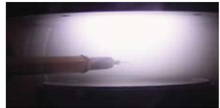
**A mysterious plasmoid-mode of operation in the Gaseous Electronics Test Cell.**
