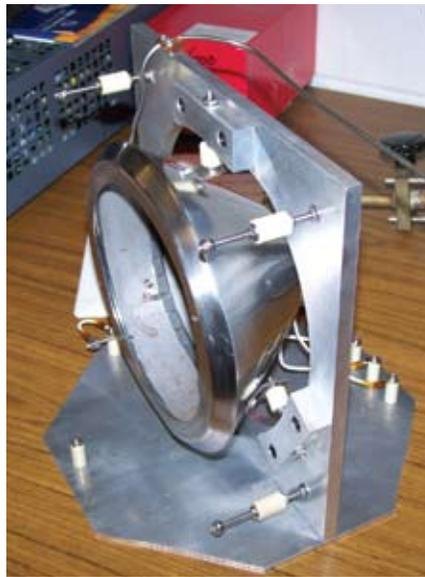
Iron thruster discharge chamber designed and built by a U-M student working in the PSTL this summer.
